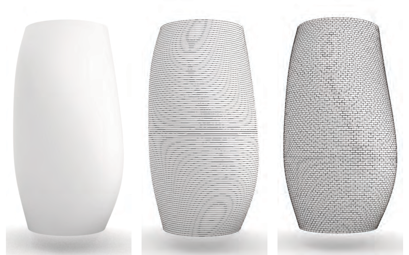
Layers of algorithmic assembly logic on doubly curved surface
